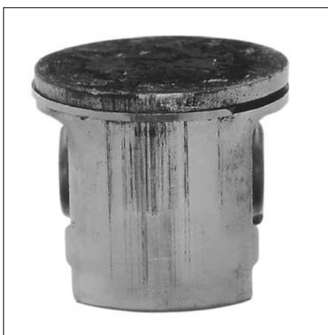
The exhaust side damaged by a broken piston ring. The piston ring parts damage the head part of the piston and result in scratch marks.
