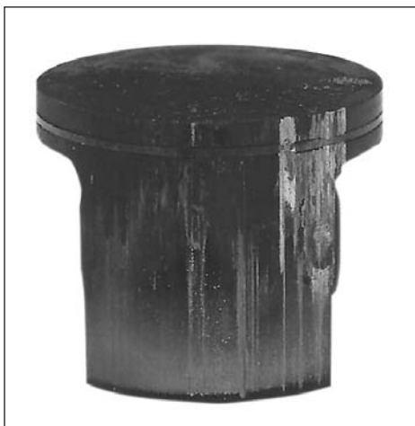
Medium to deep scratches on the exhaust side. The piston ring has stuck in its groove. Black discolouring under the piston ring resulting from so-called "blow through".
