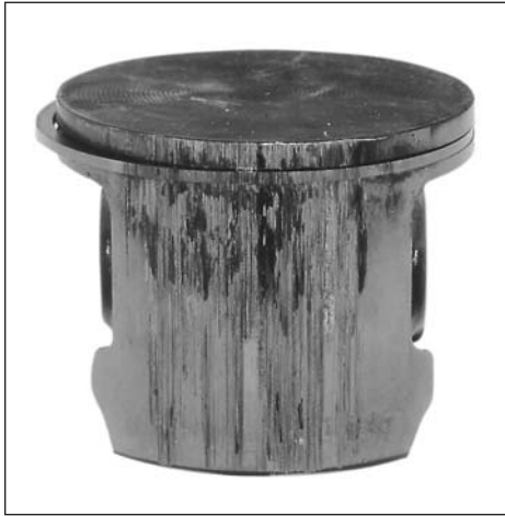
Medium sized to deep scratches along full piston skirt on exhaust side.
