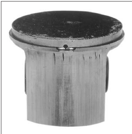
The piston is worn and scratched from the piston ring and downwards on the inlet side.
