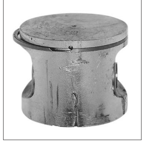
Irregular grooves on the piston's inlet side caused by a broken bearing cage.
