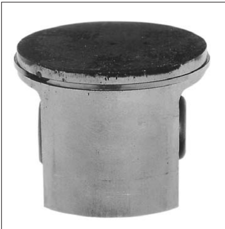
Small scratches and a dull, grey surface on the piston's inlet side resulting from fine dust particles.
