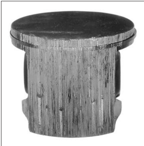
Powerful scratches along the full piston skirt on the exhaust side.
