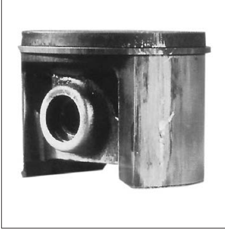
Small to medium sized scratches mainly opposite exhaust port.
